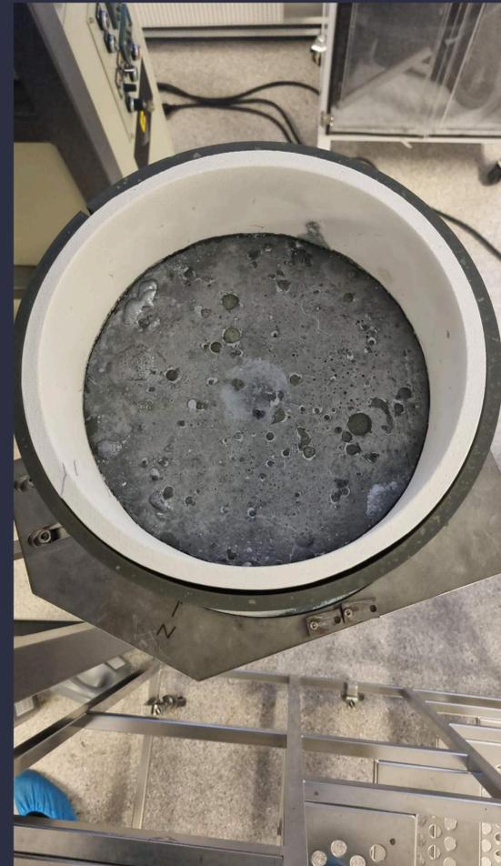
Crucible with silicon after the purification process
