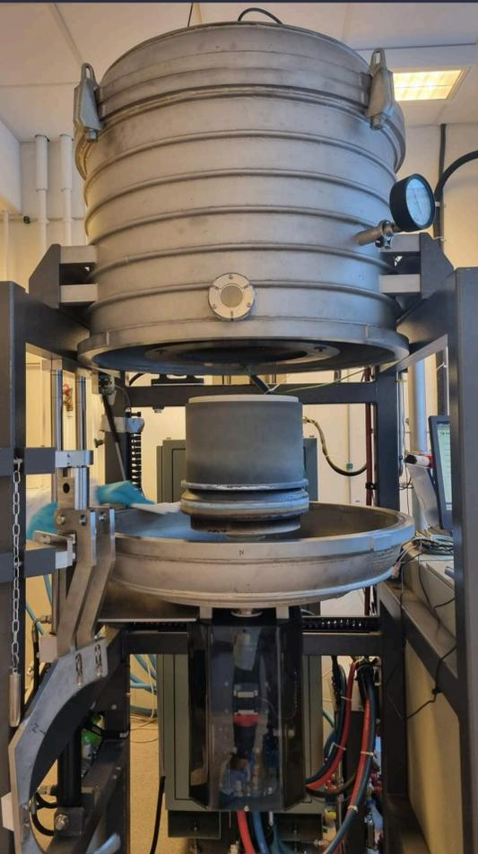
Induction heated directional solidification furnace manufactured by Crystalox Inc
