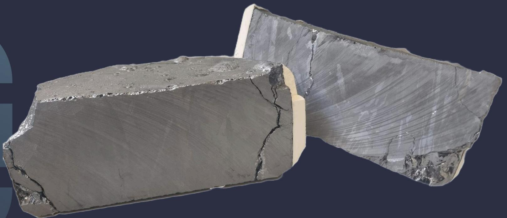
Silicon ingot made by directional solidification of silicon produced out of waste materials
