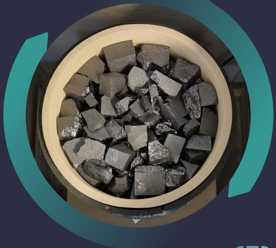
Silicon produced out of waste materials and prepared for purification experiment
