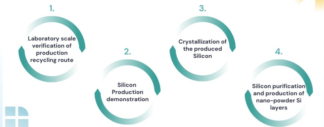
In order to reach this goal, NTNU will work on demonstrating a circular process to produce high purity silicon through aluminothermic reduction of quartz fines, followed by refining of the produced metal utilizing kerf, originating from the cutting wire during wafering of Silicon and representing a loss of more than 40 % of silicon during the process. Another innovation of this demonstration is the reuse of silicon waste from end-of -life PV modules.
