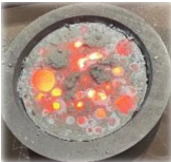
Slag tapping where metal pearls are visible on the top of casting as round pearls.
